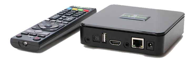
The SpotBox4K is both a H.264 & H.265 video decoder and is designed as a low cost, PC-Less way to view and display IP camera streams in Ultra high resolution onto a 4K/1080p screen or monitor.
